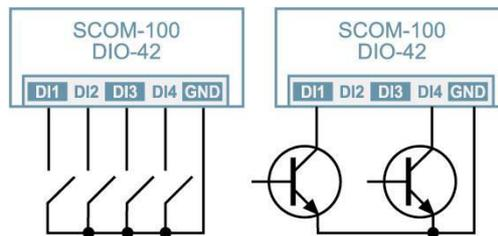
The digital inputs can be driven either by switches or transistors (open collector stages). Transducers with push-pull output are also applicable.
