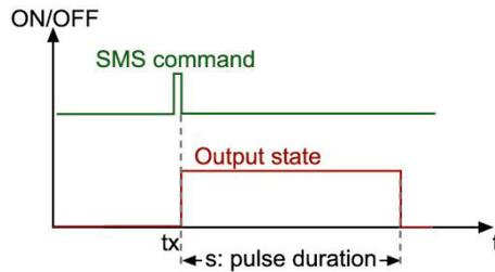
This behavior is that of a monostable timer. The command to set an output with a pulse is:
