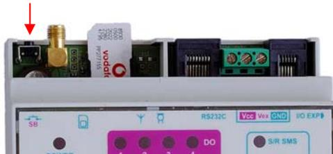
The unit executes the startup procedure setting all parameters to the factory defaults, reads the SIM card's phonebook entry, enters the RUN (Control) mode and sends a HELLO SMS message to the mobile phone number that was found in the SIM phonebook entry.
