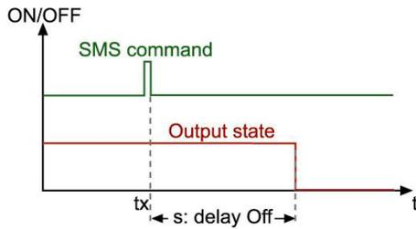
The command to reset an output after a delay is:
