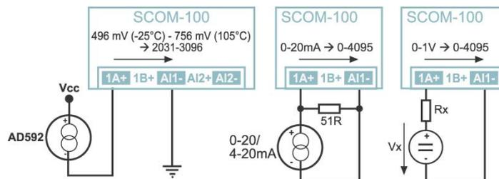
The input voltage range for this wiring option is 0-1VDC. The input resistance is 2K. The input voltage range is converted internally to a digital raw range of 0-4095.
