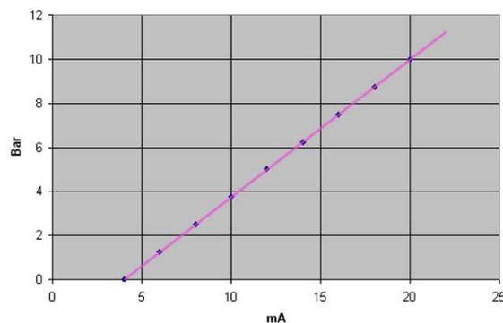
The 4-20mA input signal is converted by the internal A/D converter in the digital raw range of 819 to 4095.
