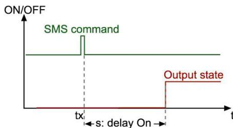
The command to set an output after an initial delay is:
