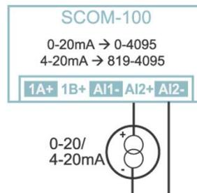
It can be used in conjunction with industry standard current loop transducers & sensors. Input impedance is 50Ω. The 0-20mA input is converted internally to a digital raw range of 0-4095.
