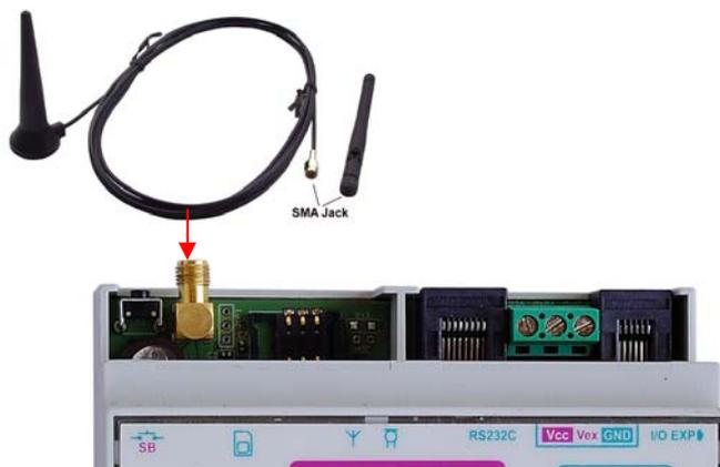
The GSM antenna must be of appropriate frequency to cover the frequency band of your GSM provider's network.
