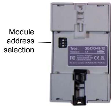
The module number (m, see sections 4.3 & 4.4) of an expansion module is determined by the DIP switch settings on the rear side of the module. The settings can be derived from the following table:
