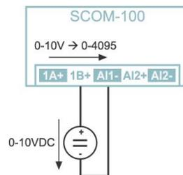
Wiring option A1B is designed for 0-10VDC signal input through an internal 18K & 2K voltage divider. The input resistance is 20K.
