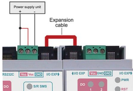
If the number of expansion modules is more than 4, an external power supply source must be connected to the power connector screw terminals of each expansion module, as shown below, and the Vcc to Vex on the main SCOM-100 unit must not be bridged.
