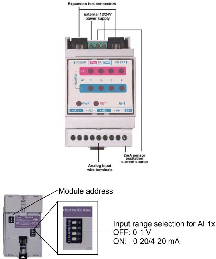
The input range of each analog input can be selected between 0-1V (DSW OFF) and 0-20mA (DSW ON) by means of the quad dip switch on the rear panel.
