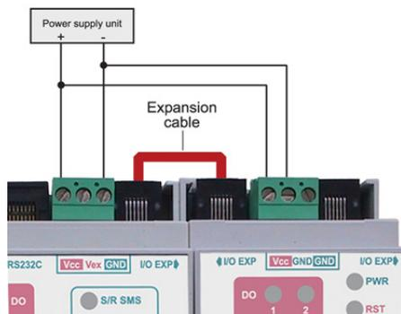
**Note:** The Vex pin must not be connected when an external power source is connected on the expansion modules because the main SCOM-100 unit will be damaged.
