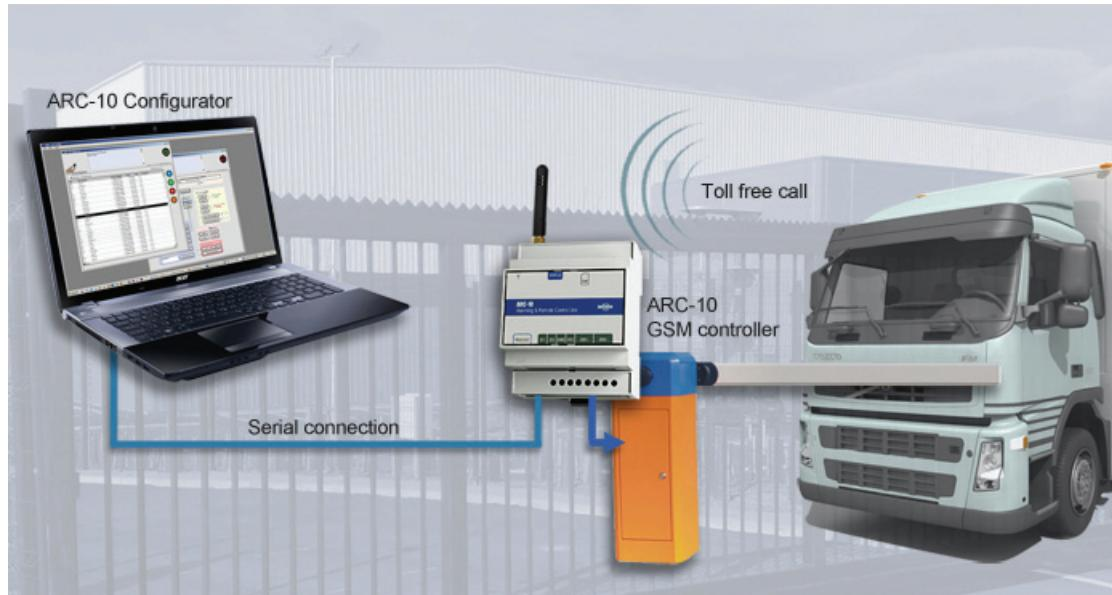
Infinite ARC-10 GSM controller provides a secure entrance access by receiving a toll free phone call from a registered user. A special contact, connected to an ARC-10 digital input, can initiate an SMS alert to security personnel, in case of a tamper attempt. Up to 10 power users can be qualified to control (enable or disable) the gate accessibility via SMS and receive alerts from the unit.
