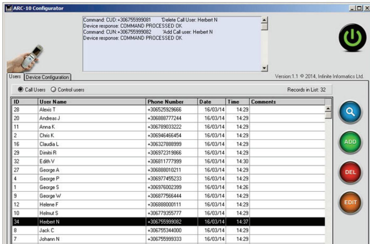
ARC-10 Configurator synchronizes every modification of a database record with the corresponding entry in the ARC-10 memory. In the above illustration, a user's phone number, which was previously edited in the database, is synchronized, by automatically executing the following 3 steps:
